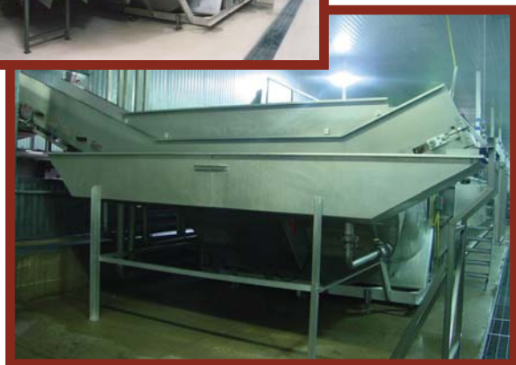
MICHIGAN TURKEY PRODUCERS, CHILLERS, BEFORE (LEFT) AND AFTER (BELOW) THEIR WATER-SAVING MODIFICATIONS
